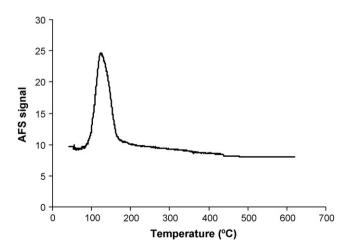
Fig. 2. Thermal decomposition profile of FGD-gypsum sample obtained with the Procedure 1.
