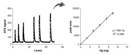
Fig. 4. External calibration (regression line) for different quantities of mercury injected in the thermal dissociation rig.
