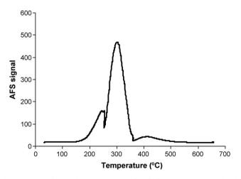
Fig. 3. Example of thermal decomposition profile of a fly ash sample obtained with the Procedure 2.
