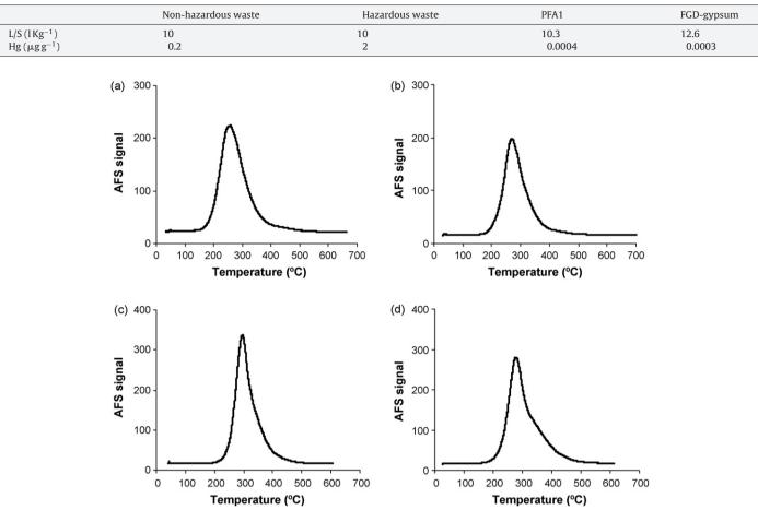
Fig. 1. Thermal decomposition profiles of (a) PFA1, (b) PFA2, (c) PFA3 and (d) PFA4 fly ash samples obtained with the Procedure 1.
